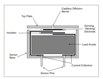
Figure 3 – Schematic of oxygen sensor.
