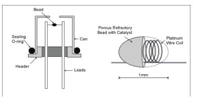
Figure 1 - Catalytic beads / Pellistors
